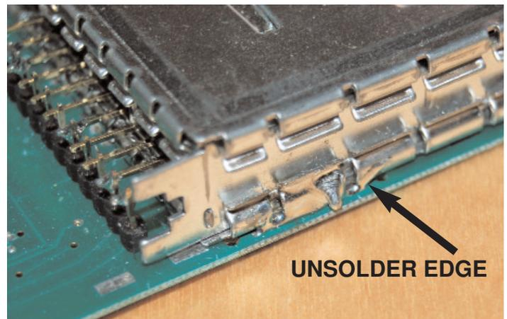
Using a small blade screwdriver gently pry up the can to break free from the board. The pins should pivot then break loose where it was soldered.
