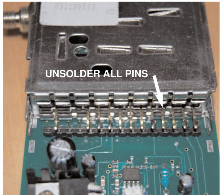
Next unsolder the two sides of the tin can where it is attached to the board, get as much solder out as you can.
