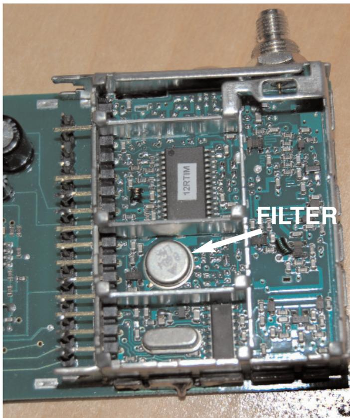
It is best to use a desoldering iron with lots of suction but wick or a manual solder sucker can do it as well. Unsolder the input and output pins (the outer ones) first. Make sure the leads are clear and no longer soldered to the board.
